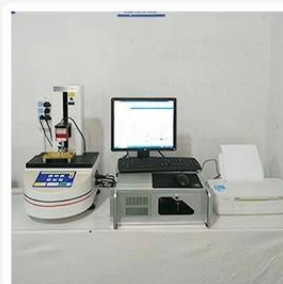
3. Load Curve Meter
