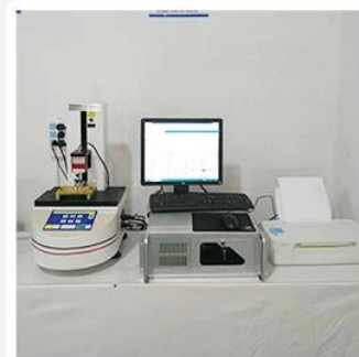
3. Load Curve Meter
