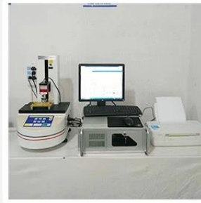
3. Load Curve Meter
