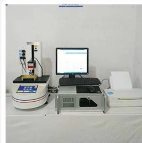
3. Load Curve Meter
