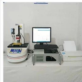
3. Load Curve Meter
