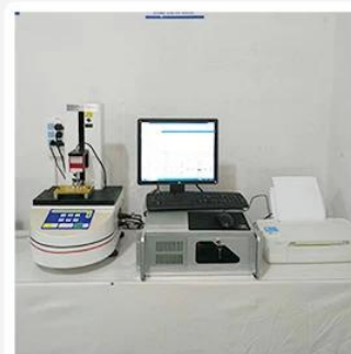
3. Load Curve Meter
