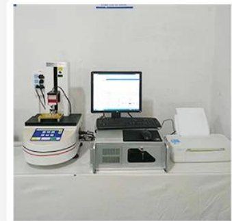
3. Load Curve Meter
