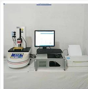
3. Load Curve Meter
