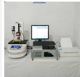
3. Load Curve Meter
