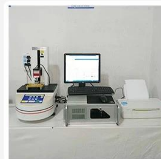
3. Load Curve Meter
