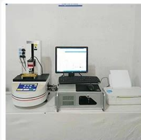
3. Load Curve Meter
