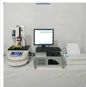
3. Load Curve Meter
