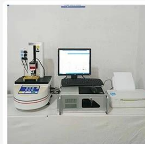
3. Load Curve Meter
