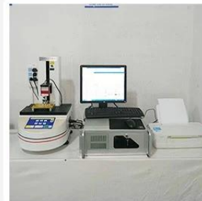
3. Load Curve Meter
