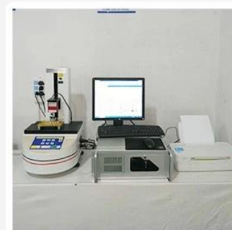
3. Load Curve Meter
