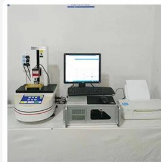
3. Load Curve Meter
