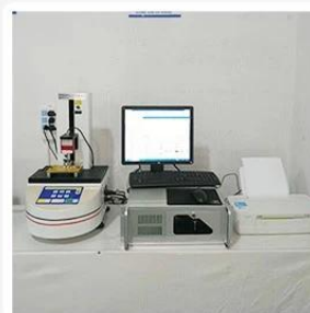
3. Load Curve Meter
