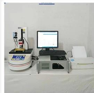
3. Load Curve Meter
