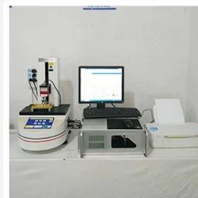
3. Load Curve Meter
