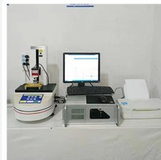
3. Load Curve Meter
