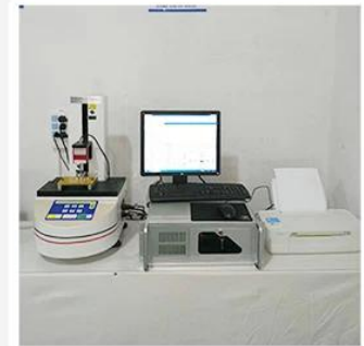
3. Load Curve Meter
