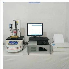
3. Load Curve Meter
