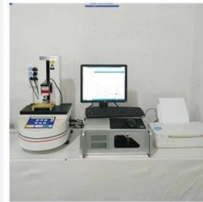
3. Load Curve Meter
