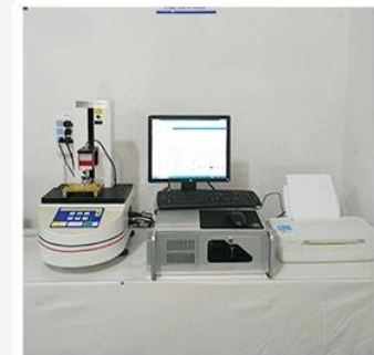
3. Load Curve Meter
