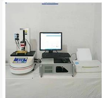
3. Load Curve Meter
