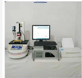
3. Load Curve Meter
