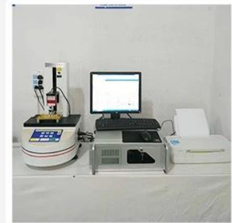
3. Load Curve Meter
