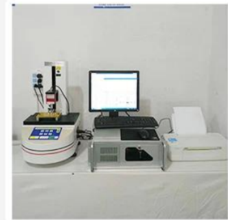
3. Load Curve Meter
